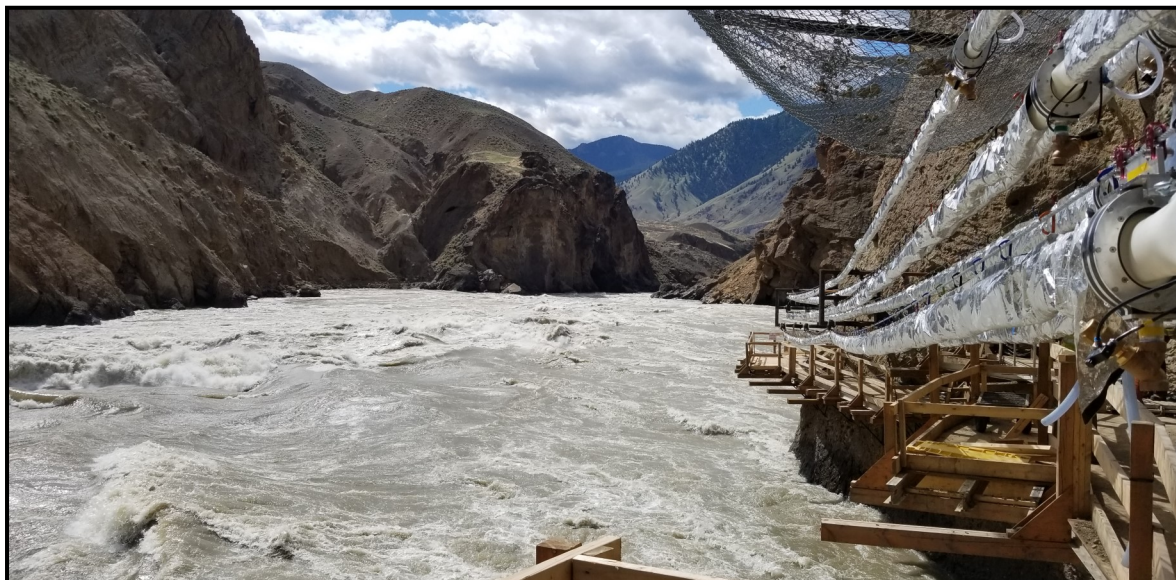
PICTURED: Whooshh™ tubes and working platform overlooking the Fraser River.
